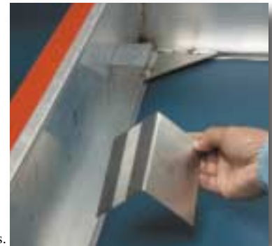
Permanently attach brackets and stiffeners.
