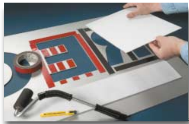
Easily cut to size, 3M™ VHB™ Tape 5952 bonds polycarbonate sheets to the back of a routed aluminum face. Surface is simply cleaned prior to application. Tape is pressed with a roller for optimum bonding.
